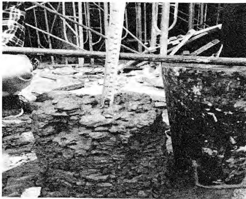
Gambar 16: Uji Slump Test
