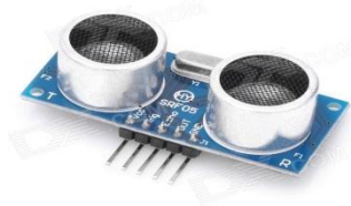
Gambar 2.7: Sensor jarak Ultrasonic HY-SRF05 Sumber : https://widuri.raharja.info/index.php/SII233473132
