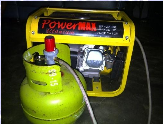
Gambar 2.20 Genset Berbahan Bakar Gas LPG.
