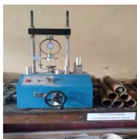
Unconfined Compression machine
