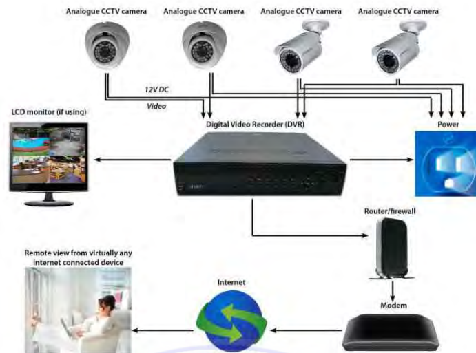
Gambar 5. 19 (CCTV) Closed-Circuit Television
