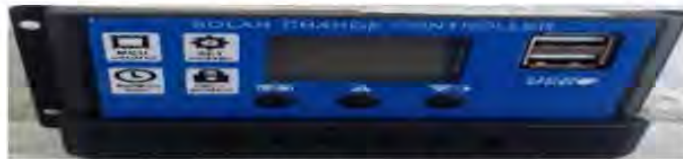
Gambar 3. 3 Solar Charger Controller
