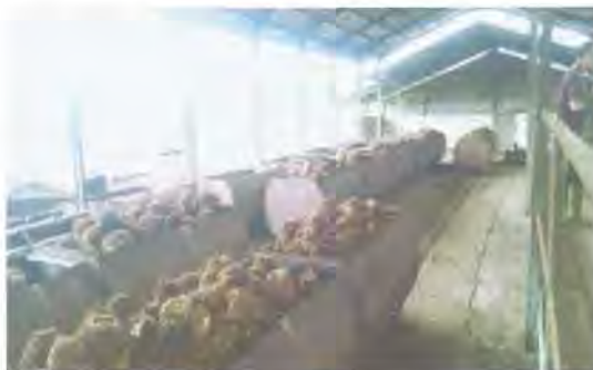
Gambar 3.6 Cage Fruit (Lori Rebusan)
