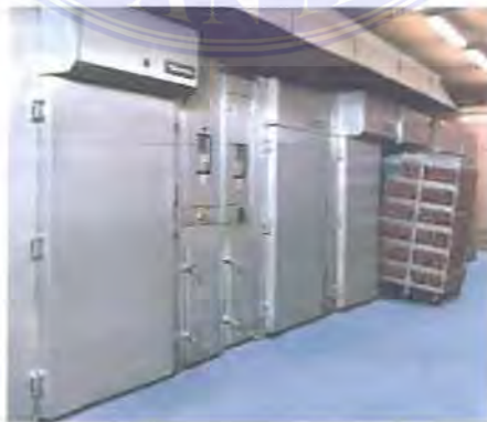
Gambar 3. 7 Smoke House Machine
