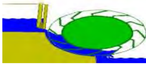
Gambar 2. 3. Kincir Air Tipe Breastshot.
