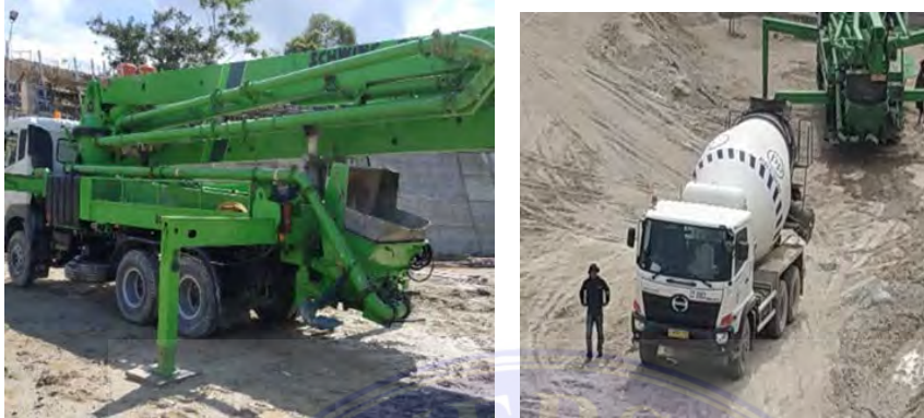
Gambar 4. 12 concrete pump and mixer truck.
