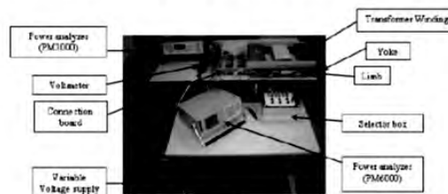
Fig. 4. Test circuit for localised flux distribution measurement
