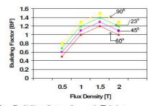
Fig. 5: Building factor for each T-joint
