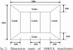
Fig. 2: Dimension (mm) of 100kVA transformer model
