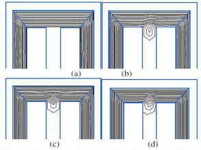
Fig. 6: Variation of magnetic flux lines in transformer core built M5 material use Software with ωt=0 (a) T- joint 90°, (b) T-joint 23°, (c) T- joint 45° and (d) T-joint 60°
