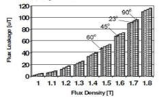
Fig. 7: Flux leakages at T-joint
