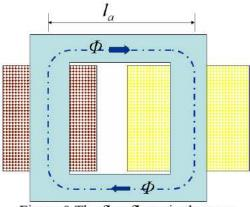
Figure 8 The flux flows in the core
