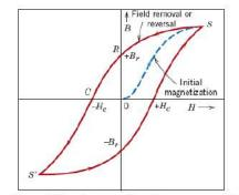
Figure 1 The B vs. H behavior for ferromagnetic material [6]
