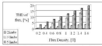
Figure 6 Total harmonic distortion of transformer under different limb
