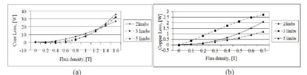
Figure 5 (a) Core loss and (b) Copper loss of transformer under different limb
