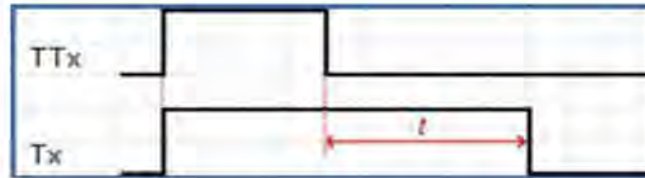
Gambar 2.10: Timing diagram timer function C: Off Delay
