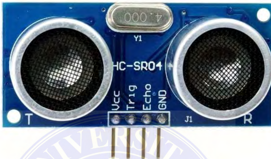
Gambar 2. 4: Sensor Ultrasonik HC – SR04. [ https://www.tokopedia.com ]
