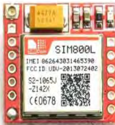
Gambar 2. 6 : Modul GSM Sim 800L. [ https://nettigo.eu ]
