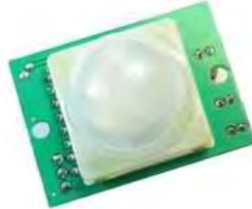
Gambar. 2.7 : Sensor Gerak Pir ( pasive infra red )
