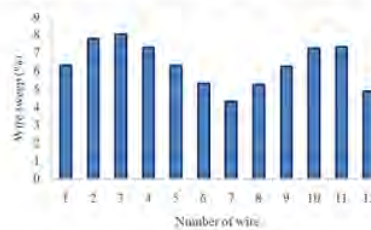
Fig. 9. Percentage of wire sweep for all wires of simulation optimization result.
