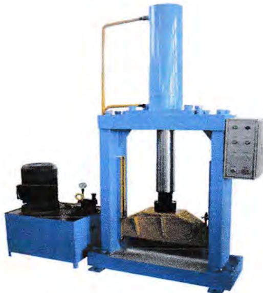
Gambar 3.1 Rubber Bale Cutting
