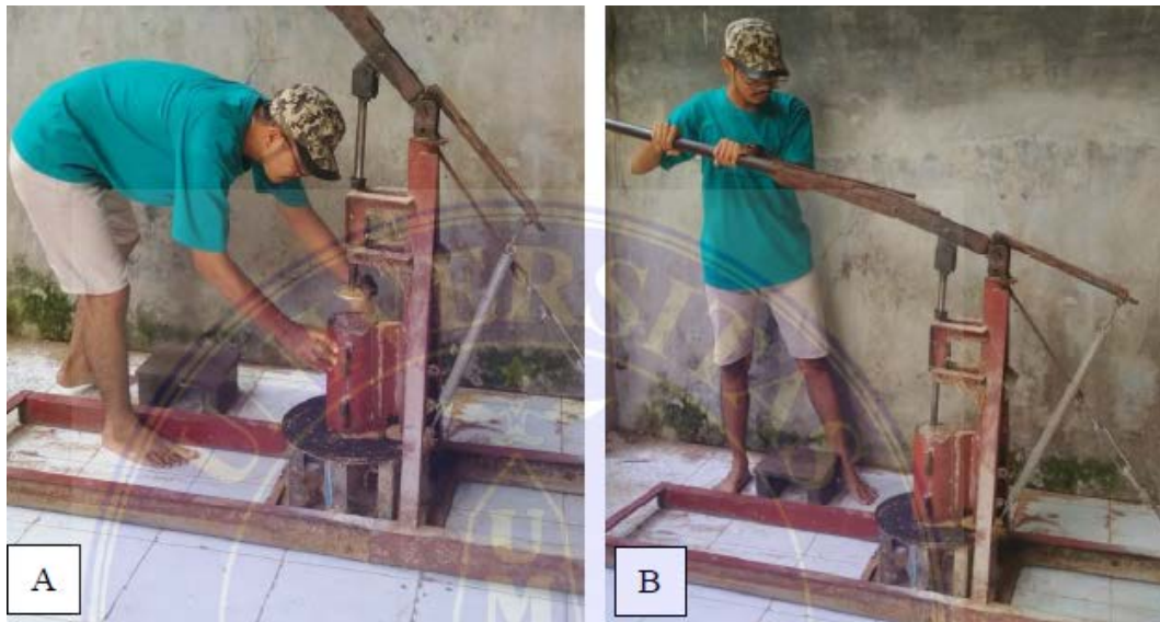
Figure 5. Pressing the Planting Media of White Oyster Mushroom into Baglog, Description: A. Laying Baglog on Pressing Equipment, B. Pressing is done on Planting Media into Baglog.
