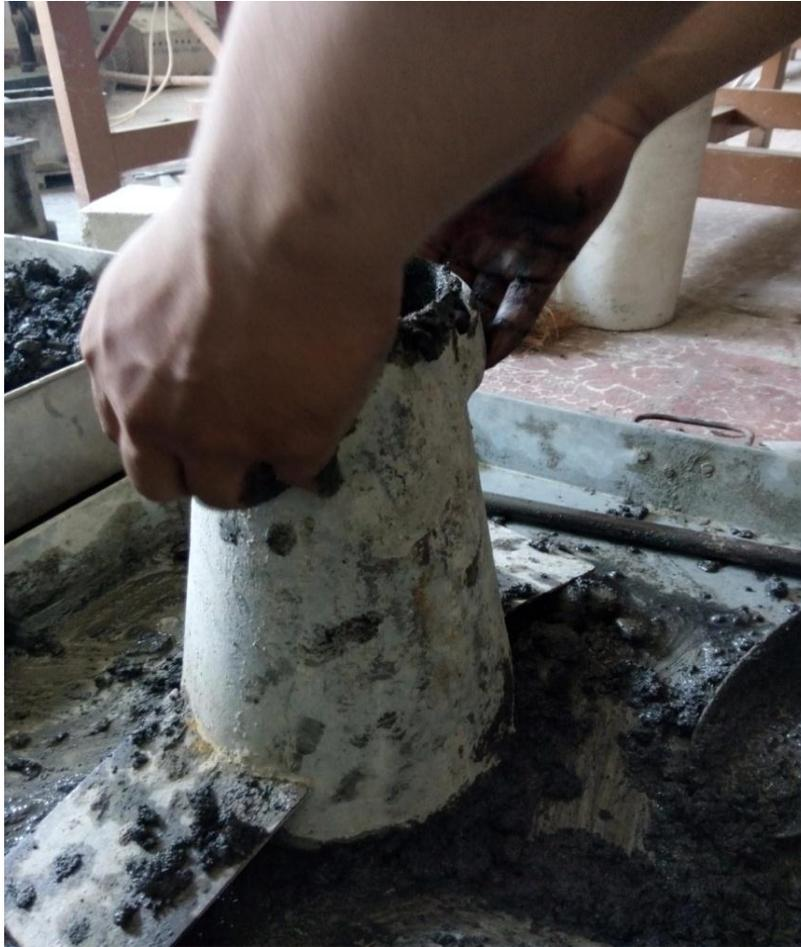
**Gambar 2.4 Slump test**
